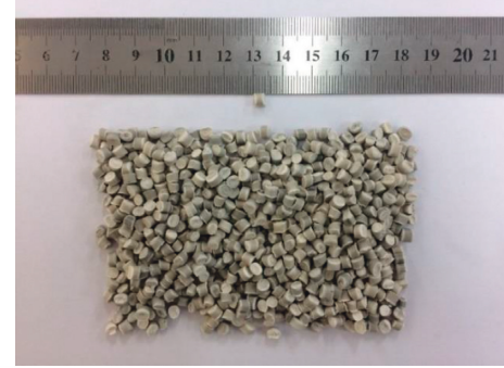
FIGURE 1: Recycled PP plastic particles with lengths from 2 mm to 3.5 mm.
