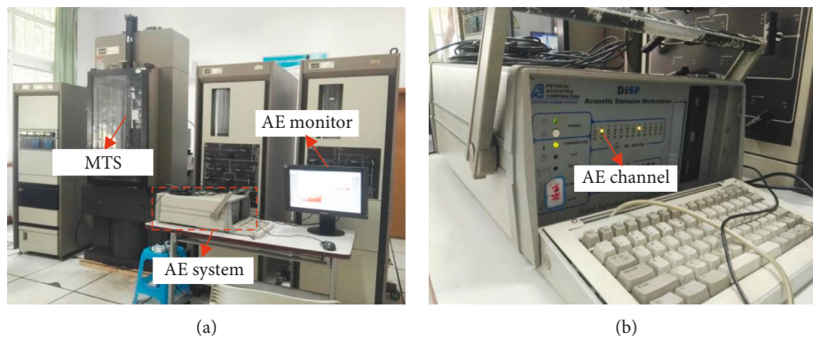
FIGURE 2: The experimental equipment. (a) MTS815 equipment. (b) 12CHS PCI-2 AE system.
