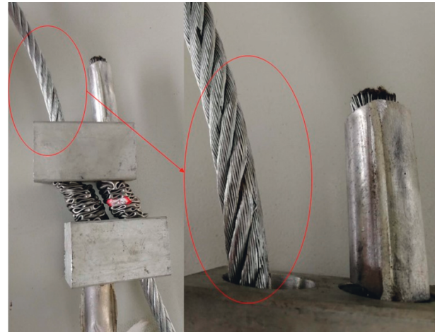
FIGURE 20: Abrasion of steel cables for tube-crushing dissipators after tests.
