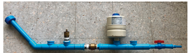
FIGURE 7: HRP body with diaphragm tank.
