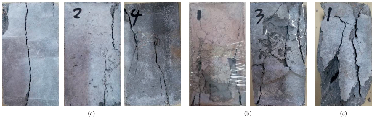
FIGURE 15: Crack morphology of specimens at different relative higher temperatures. (a) t = 100^{\circ}\text{C} . (b) t = 200^{\circ}\text{C} . (c) t = 300^{\circ}\text{C} .
