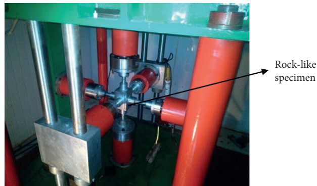
FIGURE 9: The triaxial loading machine for rock-like specimen.
