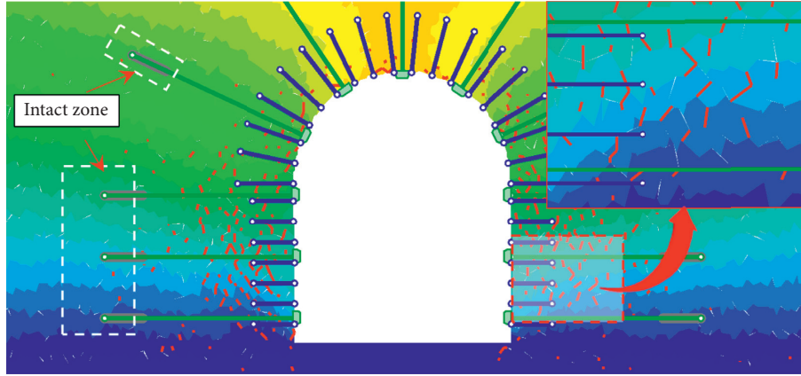
FIGURE 2: Crack development characteristics of the chamber.
