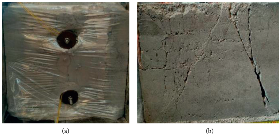
FIGURE 9: Diagram of fragmentation of two rockbolts. (a) Frontal destruction. (b) Side destruction.
