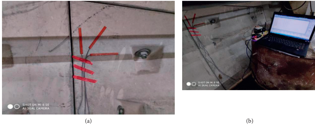
FIGURE 18: Site monitoring chart. (a) Layout of strain gauges. (b) Data acquisition of static monitor.
