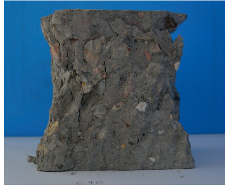
FIGURE 5: Axial compression failure mode image of concrete.
