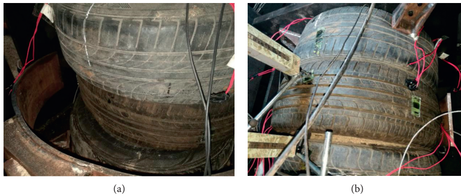
FIGURE 13: Failure state of specimen SD-8. (a) Misalignment between tires. (b) Sand leakage.
