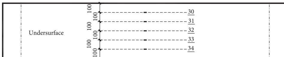
FIGURE 5: Arrangement of steel plate strain gauges.
