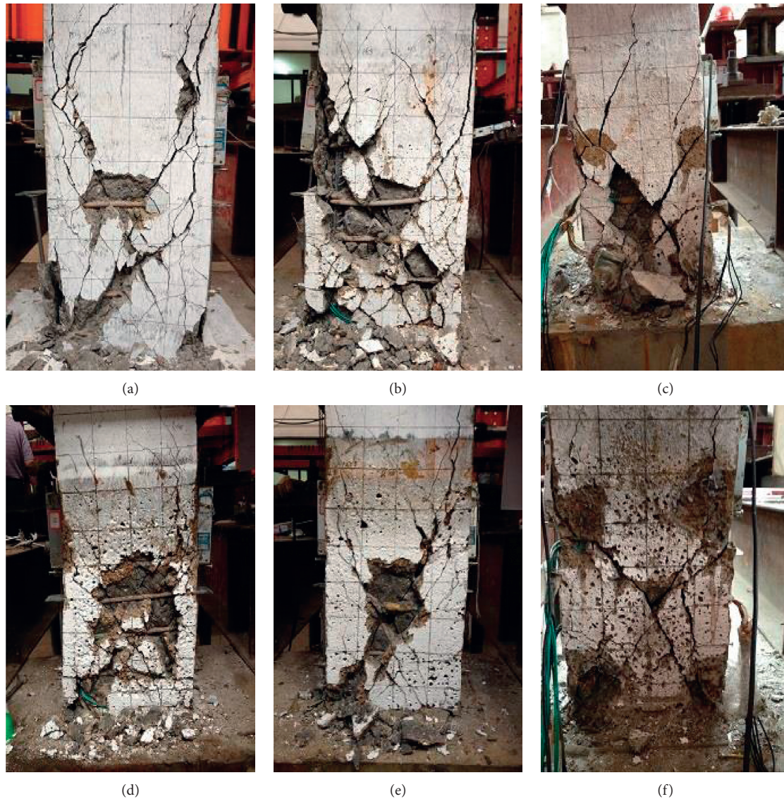
FIGURE 6: Ultimate crack patterns and failure morphologies of the specimens: (a) SC-1; (b) SC-2; (c) SC-3; (d) SC-4; (e) SC-5; (f) SC-6.
