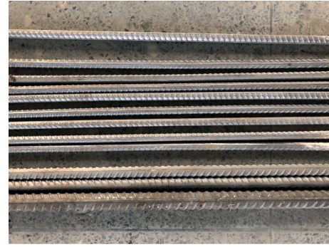
FIGURE 1: Stainless steel reinforcement.
