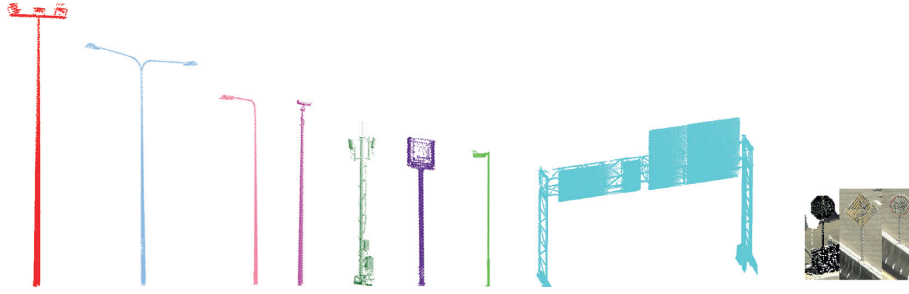
FIGURE 10: Expressway facilities being classified (from left to right) as high-mast lighting, lighting pole-2-sided, lighting pole-1-sided, CCTV camera, telecommunication tower, speed limit pole, lighting pole-1-sided (special type), overhead sign, and some types of small signboards.
