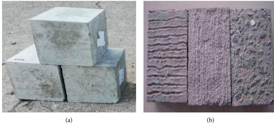
FIGURE 4: Standard model of concrete test block. (a) Test blocks of 150 mm \times 150 mm \times 150 mm. (b) Test blocks of 150 mm \times 150 mm \times 300 mm.
