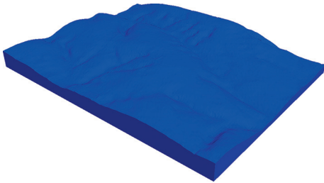
FIGURE 6: Three-dimensional model generated by a hexahedral element above an elevation of 883 m.
