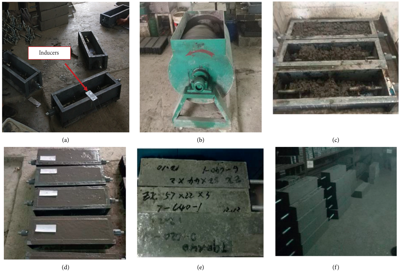
FIGURE 2: Flow chart of RCC specimen fabrication, (a) assembly, (b) mixing, (c) charging, (d) trowel finish, (e) form removal, (f) maintenance.
