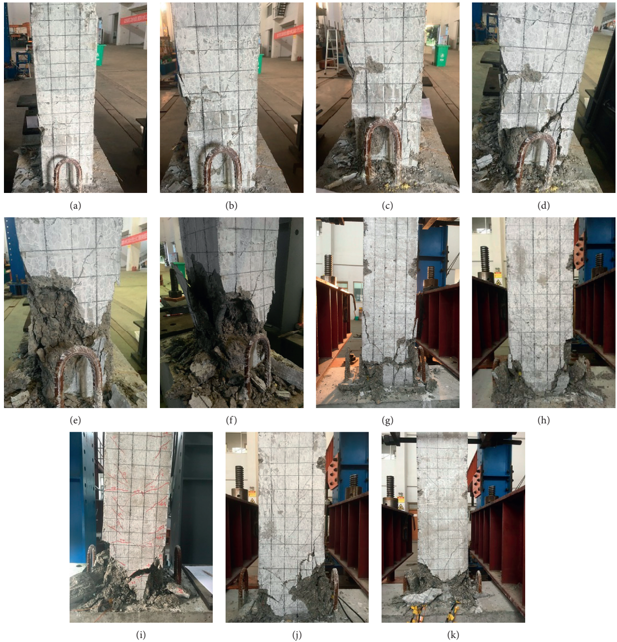
FIGURE 3: Failure mode of specimens. (a) SRC4 (1.5%). (b) SRC4 (2.0%). (c) SRC4 (2.5%-1st). (d) SRC4 (2.5%-6th). (e) SRC4 (2.5%-10th). (f) SRC4 (failure). (g) SRC1. (h) SRC2. (i) SRC3. (j) SRC1-2. (k) SRC4-2.
