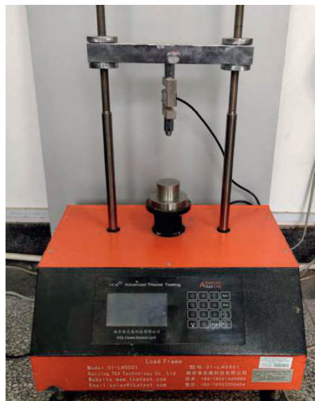
FIGURE 3: The unconfined compressive strength test machine.
