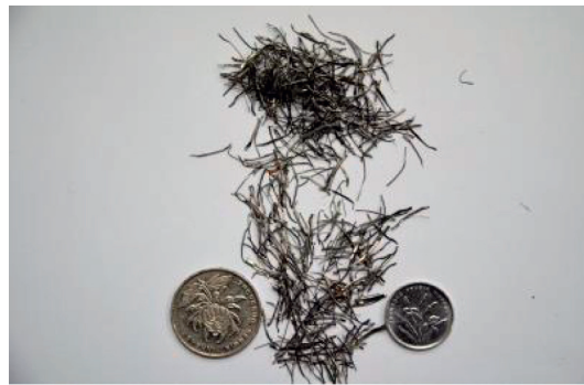
FIGURE 4: Type II (deformed cut sheet) microsteel fiber.
