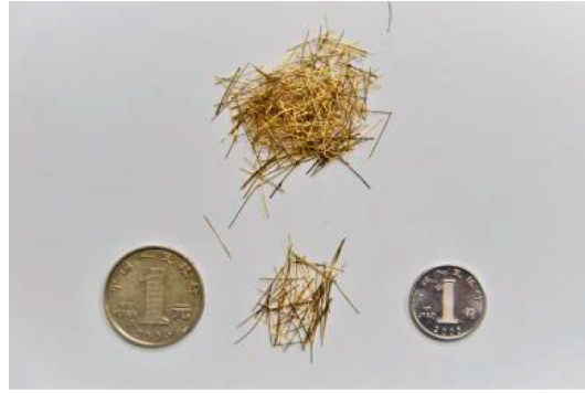
FIGURE 3: Type I (smooth cold-drawn wire) microsteel fiber.
