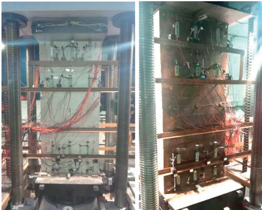
FIGURE 22: Field displacement meter arrangement for compressive experiment.
