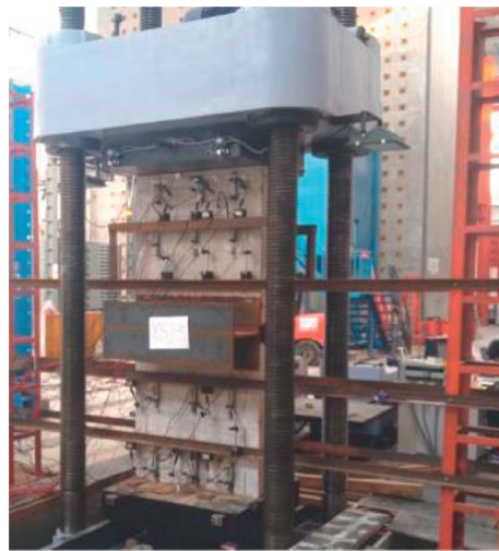
FIGURE 20: Field loading and testing of the compressive experiment.
