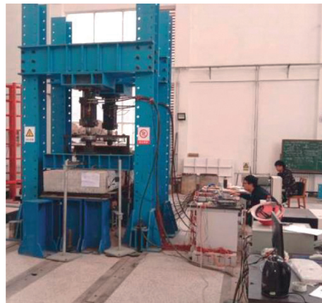
FIGURE 8: Field loading and testing of the flexural experiment.
