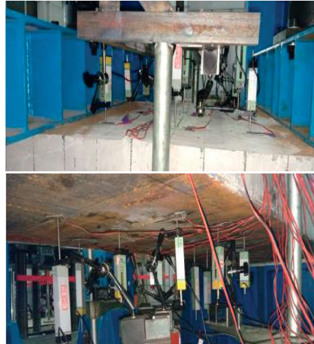
FIGURE 10: Field displacement meter arrangement of flexural experiment.
