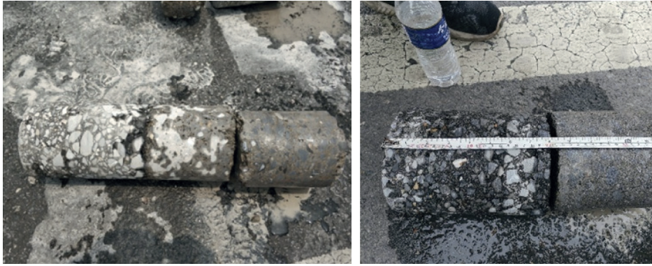
FIGURE 7: On-site sampling of asphalt pavement.
