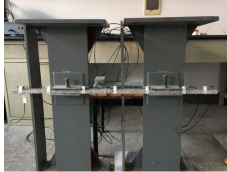
FIGURE 1: The sensors network layout for the rod-shaped rock samples.
