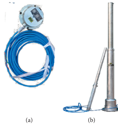
FIGURE 10: Monitoring instruments and implementation plans. (a) Filling body stress monitor. (b) Roof dynamic monitors.
