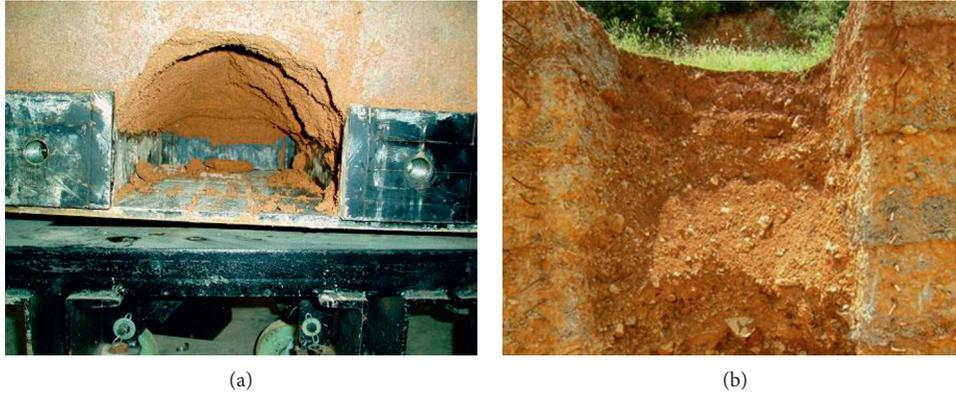
FIGURE 2: Pile-side soil arch destruction. (a) Laboratory test. (b) Practical engineering.
