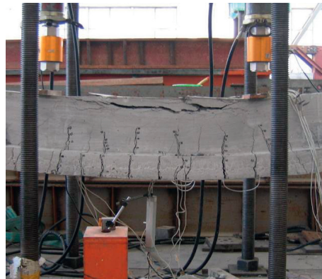
FIGURE 12: Cracked test beam SCB-1.
