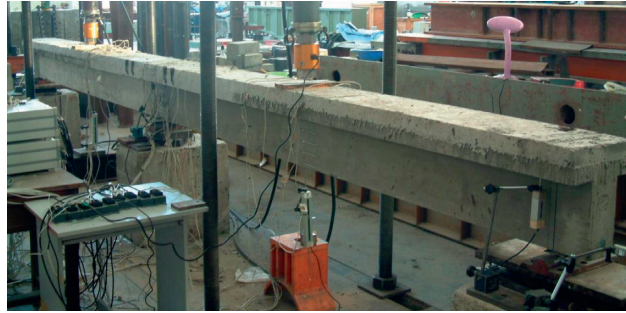
FIGURE 11: Two-span continuous composite T-shaped beam actual test setup.
