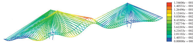
FIGURE 27: Structural displacement after repair (unit: m).
