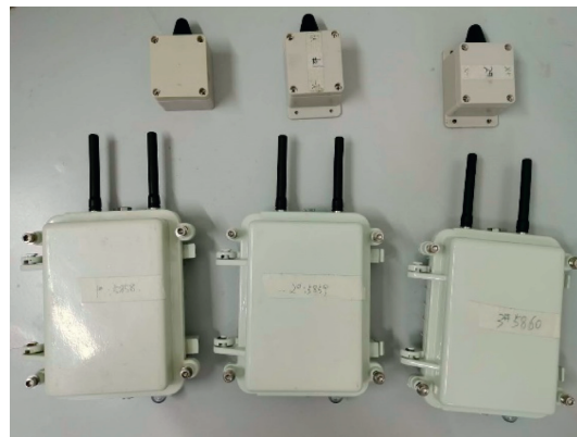
FIGURE 3: Photograph of the inclinometers and data acquisition and transmission devices.
