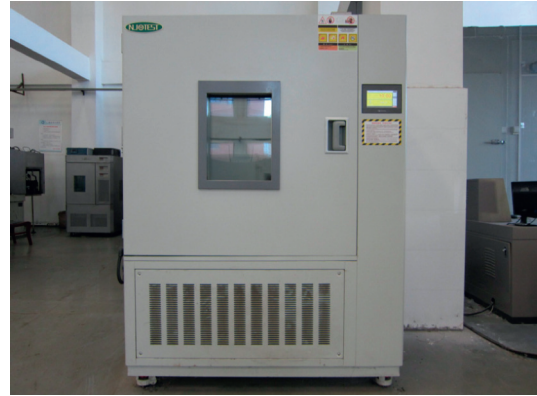
FIGURE 1: Freezing and thawing cycle test freezing room.
