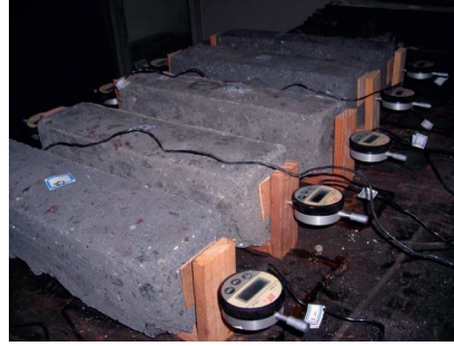
FIGURE 3: Schematic diagram of the shrinkage test.
