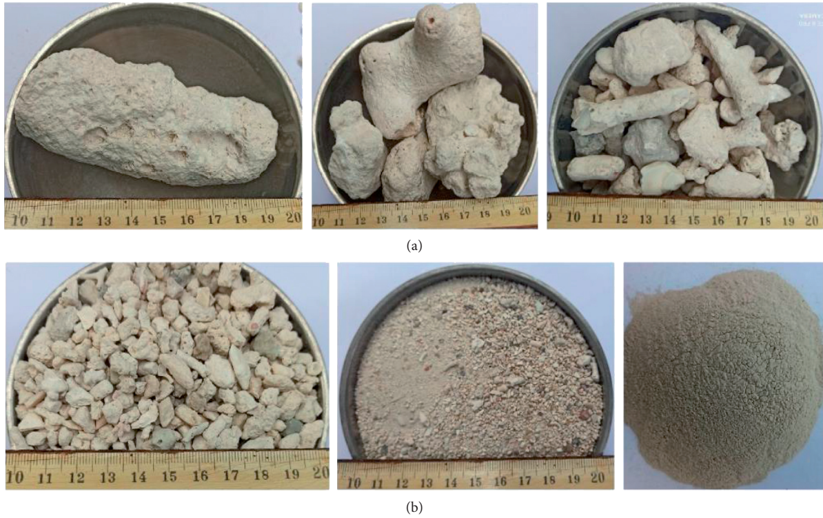
FIGURE 1: Calcareous sand samples with different particle sizes (mm).
