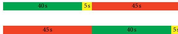
FIGURE 7: The traffic signal timing. Green time, amber time, and red time are equal to 40 s, 5 s, and 45 s, respectively.
