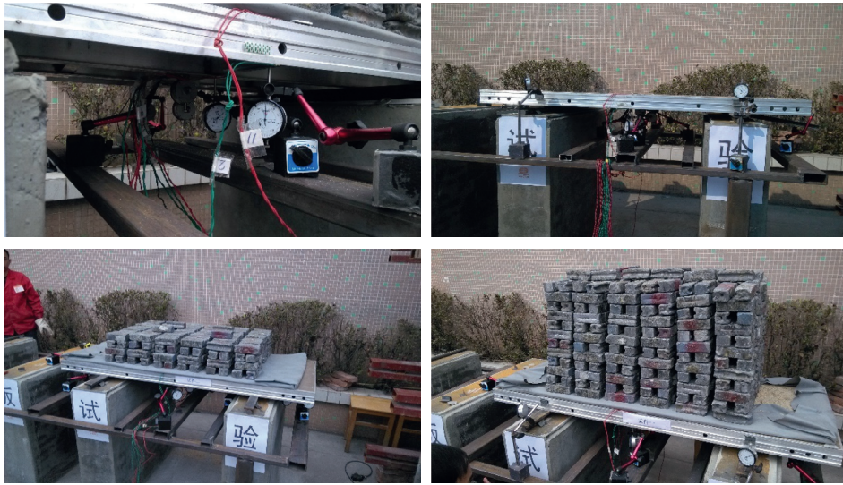
FIGURE 6: Loading process of the single-span simply supported formwork.
