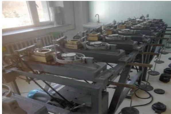
FIGURE 3: Electric strain direct shear apparatus.
