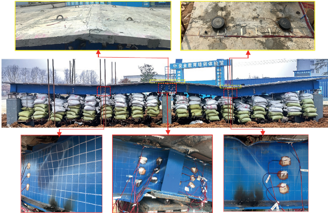
FIGURE 6: Failure mode of the model under the ultimate state (view of the internal girder).
