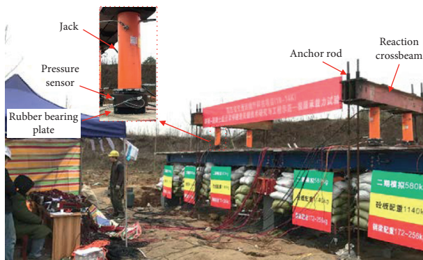
FIGURE 4: Overview of the test setup.
