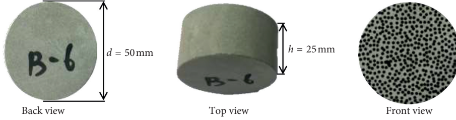
FIGURE 1: Specimens with nonvisible cracks and weak planes for Brazilian disks.
