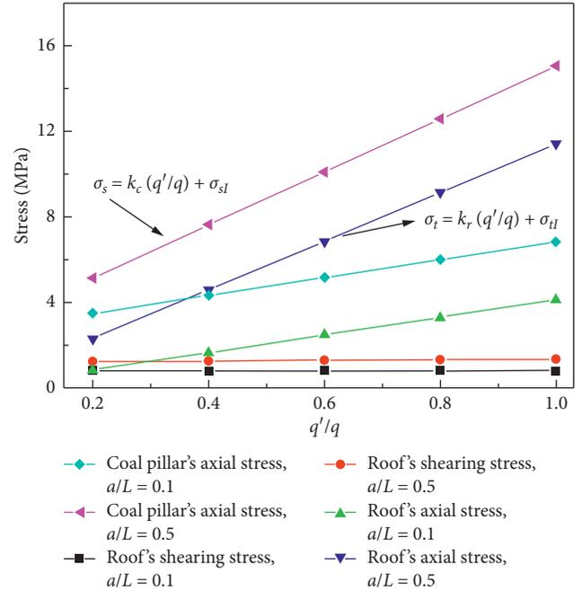
FIGURE 11: The relationship of the stress ratio  $q'/q$ .
