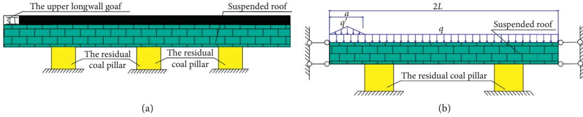
FIGURE 4: Diagrammatic figure and simplified mechanical model.
