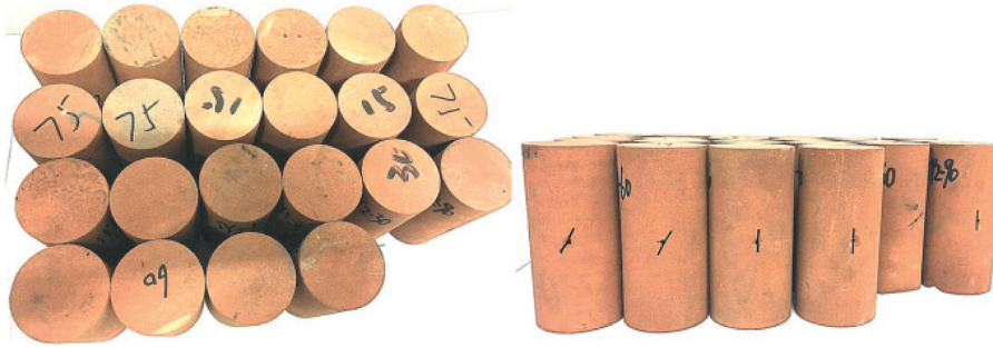
FIGURE 1: Prefabricated single-crack red sandstone specimens.
