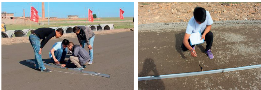
FIGURE 6: Longitudinal and horizontal evenness detection.
