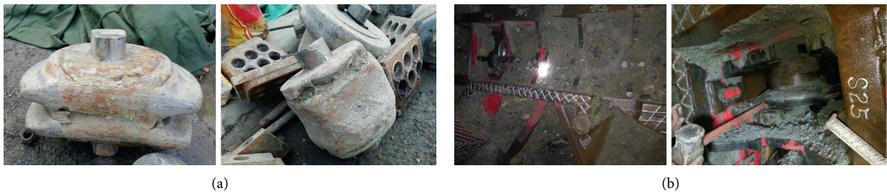
FIGURE 13: Excessive wear of the cutter tools and clogging of the cutter-head.
