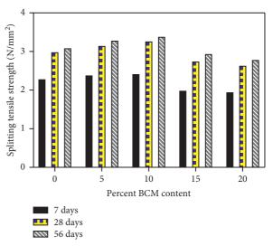
FIGURE 4: Splitting tensile strength.
