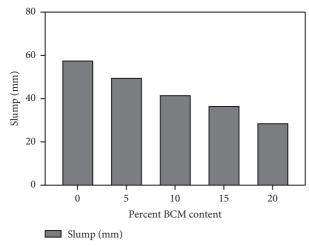
FIGURE 1: Workability of concrete.
