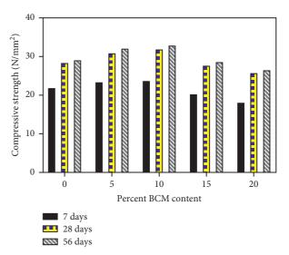
FIGURE 3: Compressive strength of concrete.
