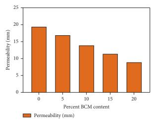
FIGURE 6: Permeability of concrete containing BCM after 28 days.
