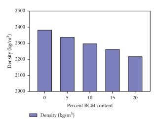
FIGURE 2: Density of concrete after 28 days.
