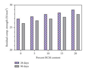
FIGURE 7: Residual compressive strength of samples exposed to chloride attacks.
