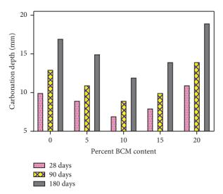
FIGURE 8: Carbonation depth of concrete containing BCM.
