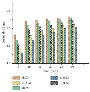
FIGURE 9: Drying shrinkage of concrete containing BCM.
