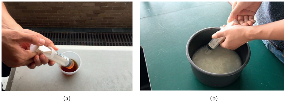
FIGURE 5: The additives used in the soil improving. (a) Tung oil. (b) Sticky rice juice.
