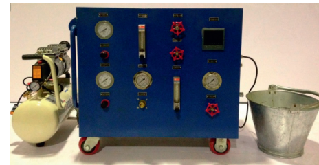
FIGURE 3: Image of foam generator.
