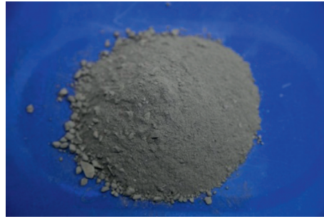
FIGURE 9: Test sample of silty sand from the tunnel site.
