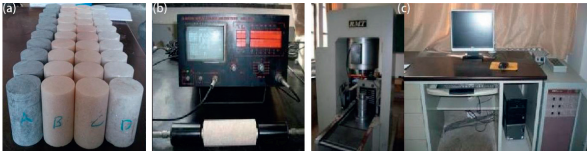
FIGURE 2: Specimen and test equipment: (a) marble specimen; (b) ultrasonic detector; (c) RMT-150B rock mechanical test system.
