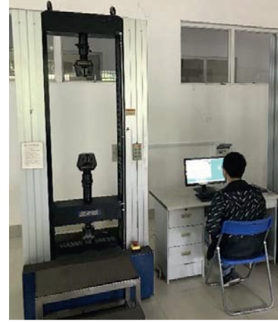
FIGURE 1: Static Brazilian test with the SANS material testing machine.
