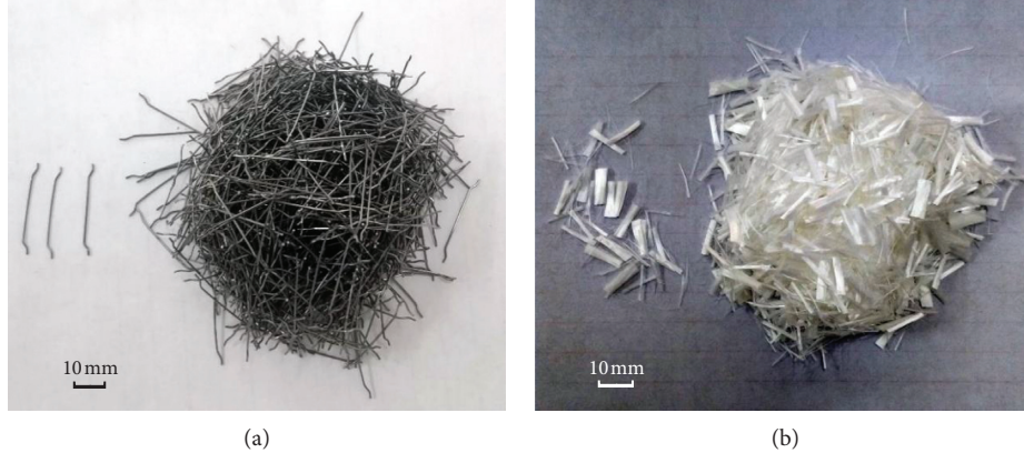
FIGURE 1: Appearance of the fibers: (a) steel fibers (SFs); (b) polypropylene fibers (PFs).
