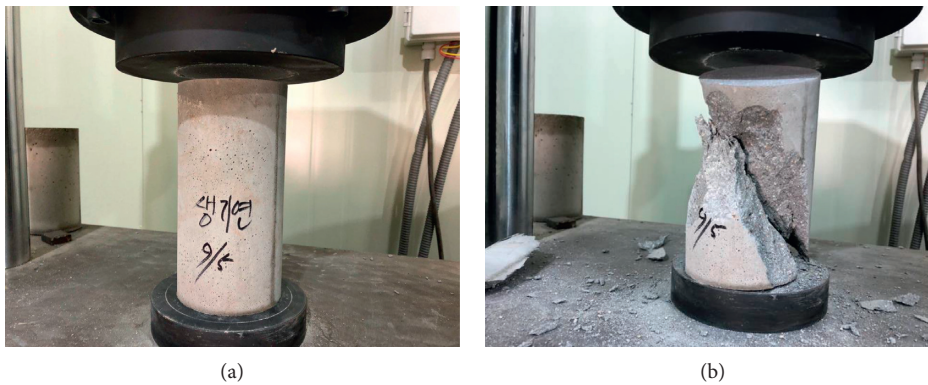
FIGURE 14: Uniaxial compression testing of a concrete specimen: (a) test setup and (b) test result.
