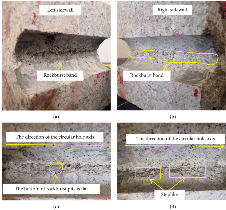
FIGURE 7: Failure characteristics of circular hole wall after rockburst.
