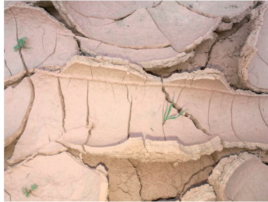
FIGURE 9: Curling of cracks observed in situ (Xi'an, Shaanxi province).
