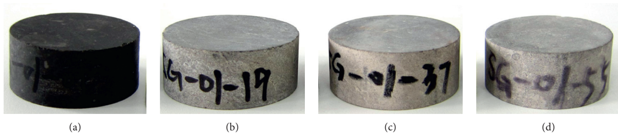
FIGURE 2: Apparent morphology of limestone specimens after high temperature. (a) 25°C. (b) 200°C. (c) 400°C. (d) 600°C.
